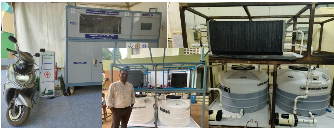
Standalone 5kW/10kWh flow battery stack (Developed with ONGC funding with industry partner High Energy Batteries I Ltd.) charging two wheeler show cased in Indi Energy Week held in Goa between 6 th -9 th February 2024
