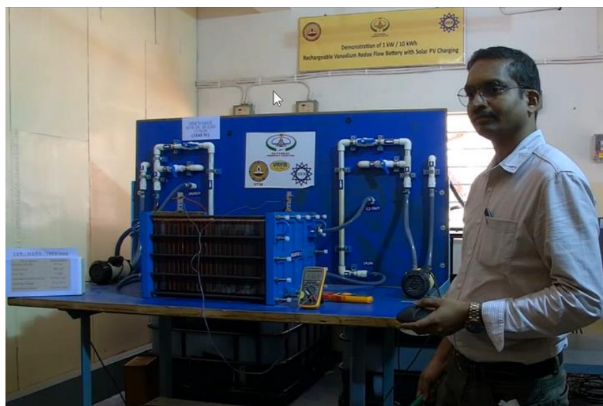
A photograph of 1.4kW/10kWh system developed with industrial partner for ONGC-Energy Trust Centre.
