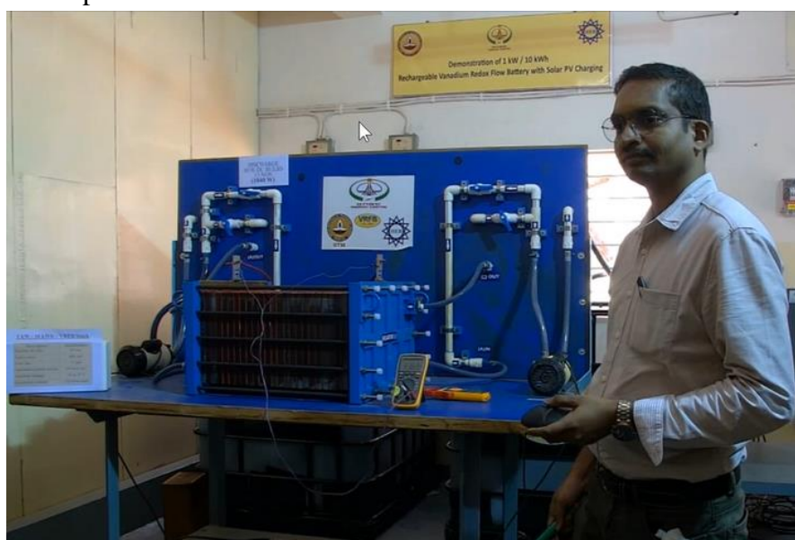
A photograph of 1.4kW/10kWh system developed with industrial partner for ONGC-Energy Trust Centre.
