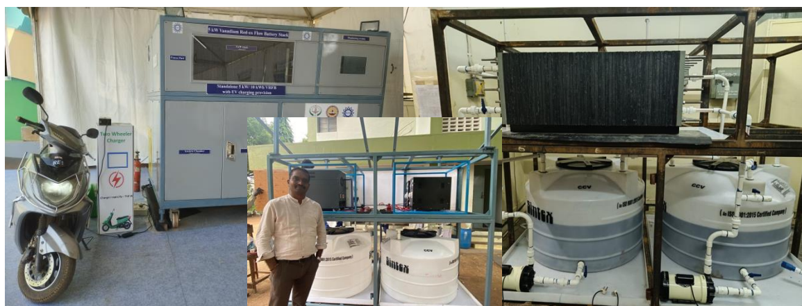
A photograph of 1.4kW/10kWh system developed with industrial partner for ONGC-Energy Trust Centre.
